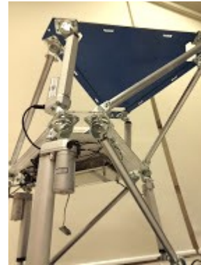
Figure 5. Table from below showing detail of linear actuator arrangement.
