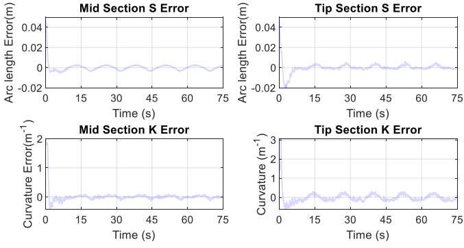
Fig. 9. Two section experiment 1 (OctArm tip and mid sections) — Arc length s , and curvature k error in configuration space.
