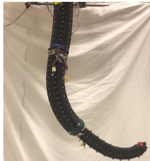
Fig. 1. Dynamically controlled OctArm, a pneumatically actuated continuum manipulator with three sections, following a desired configuration trajectory.
