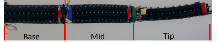
Fig. 5. The OctArm manipulator with base, mid, and tip sections.
