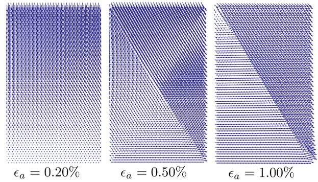
Fig. 6. Relative displacement fields at different axial strain levels for the DEM simulation.
