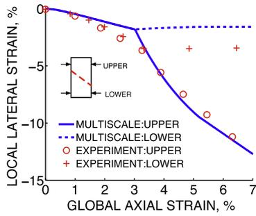
Fig. 15. Lateral strain vs. axial strain.
