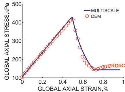
Fig. 9. Comparison of global stress–strain behavior: multiscale vs. DEM.
