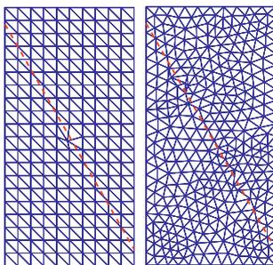
Fig. 8. Meshes used in plane strain simulations coupled with DEM.
