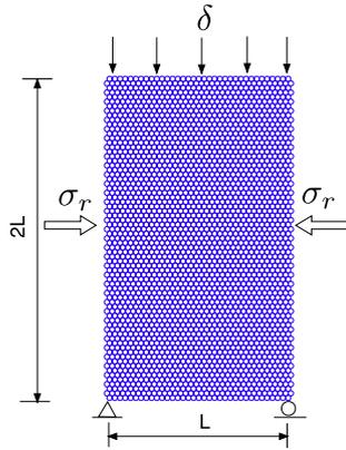
Fig. 4. Initial configuration and boundary conditions under plane strain loading of the DEM model.
