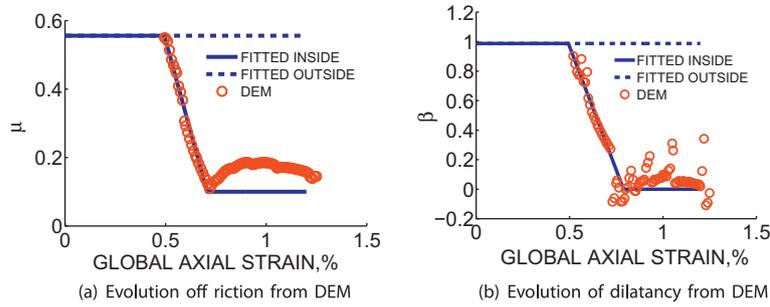
Fig. 7. Evolutions of plastic internal variables from DEM computation.
