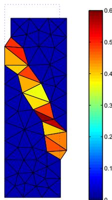
Fig. 17. Deviatoric strain contour at 7% global axial strain for mesh 3.
