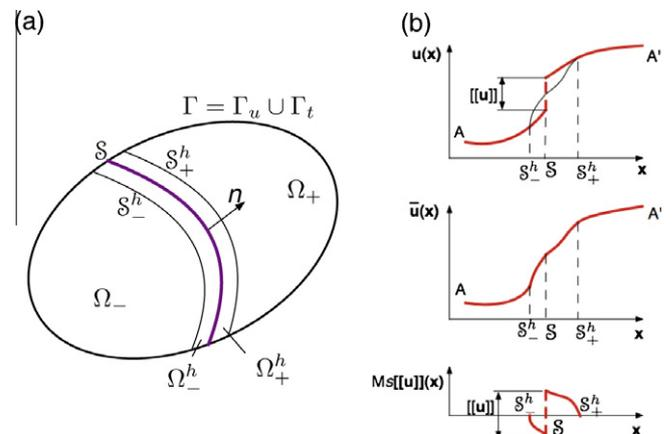
Fig. 1. (a) Domain  $\Omega$  with a surface of discontinuity  $S$ ; (b) One-dimensional representation of the decomposed displacement field.
