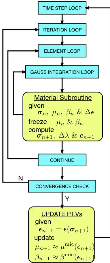
Fig. 3. Flowchart for the hierarchical multiscale scheme, modified from [44].
