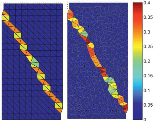
Fig. 10. Deviatoric strain contour at 1% global axial strain.
