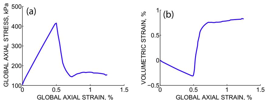
Fig. 5. Stress–strain behavior of the DEM simulation in plane strain compression test: (a) Axial stress vs. axial strain; (b) Volumetric strain vs. axial strain.
