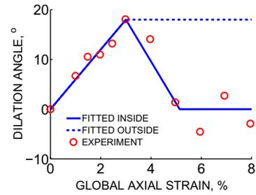
Fig. 12. Evolution of dilation angle observed in the experiment.
