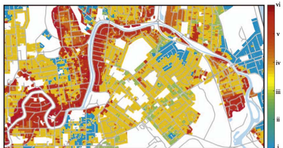
(c) Observations: i. No observed ground cracking or ejected liquefied material; ii. Minor ground cracking but no observed ejected liquefied material; iii. No lateral spreading but minor to moderate quantities of ejected material; iv. No lateral spreading but large quantities of ejected material; v. Moderate to major lateral spreading; ejected material often observed; vi. Severe lateral spreading; ejected material often observed. [42]
