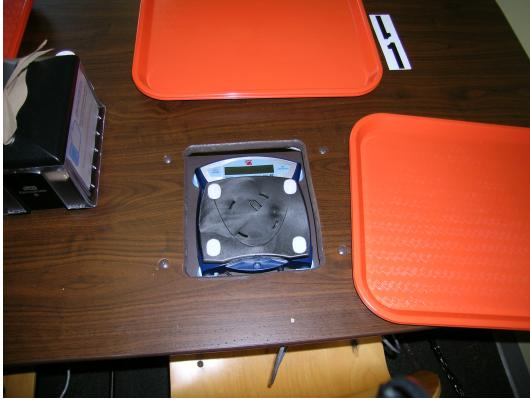
Fig. 10: A scale was mounted beneath each participant's tray.
