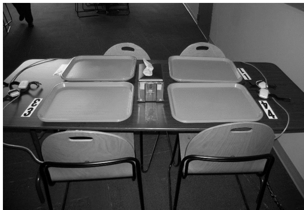
Figure 1. The instrumented table. Each station has a tethered bite counter and a camera mounted in the ceiling to record the meal.
