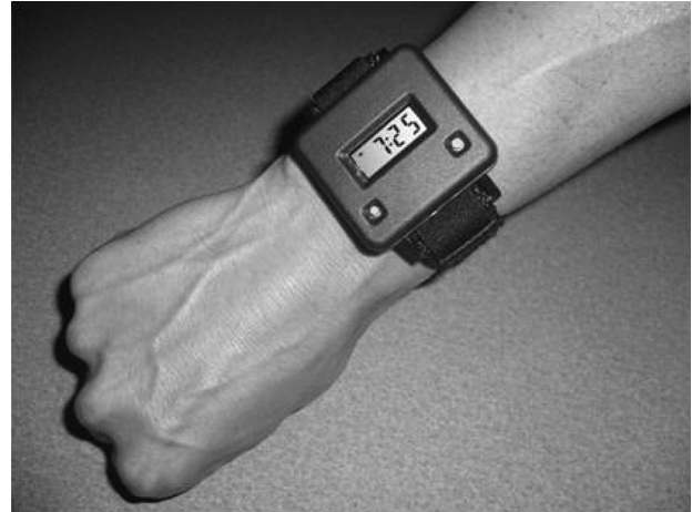
Figure 1. The bite-counting device worn on the wrist in “time” mode.
