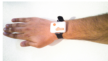
Fig. 1. Photo showing the Shimmer3 wrist mounted platform.
