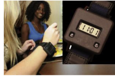
Notes: The Bite Counter™ is worn on the wrist like a watch, detects a wrist-rolling motion in order to observe that the wearer has taken a bite of food, and records a log of time-stamped bite count data in real-time. Further details can be found at www.icountbites.com .
