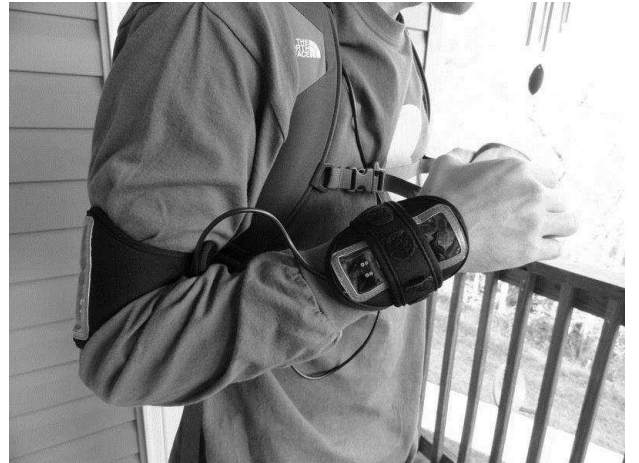
Fig. 2. Data collection using a single orientation sensor on the wrist
