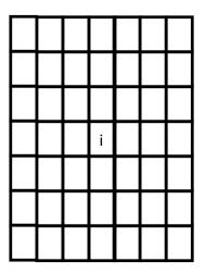
calculate energy at each pixel in window; contour point i moves to pixel with lowest energy
