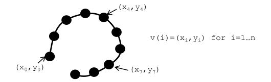
The contour is moved by searching in the neighborhood of each pixel on the contour for a better location. For example, suppose we are searching for a new location for pixel i in a 7x7 window:
