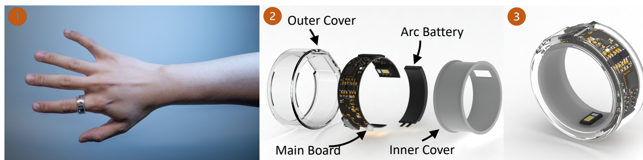
Figure 1: OmniRing is designed by integrating low-cost off-the-shelf electronic components based on SoC architecture into a flexible PCB that can bend in the form factor of a ring. IMU and PPG sensors are embedded for enabling motion analytics and healthcare applications. The hardware is enclosed in a 3D-printed waterproof case that allows smooth contact with the skin. Overall form factor weighs about 2.5 g with a week of battery life for comfortable and long-term wearing including while sleeping and swimming.
