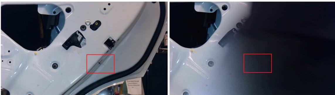
Figure 2.18: Sample images taken during the inspection process for the child safety lock use case. (From left to right) case with no occlusion; case with occlusion. The case with occlusion has also occluded the trigger, and this case (along with 7 other similar cases) will not be considered as occlusions in the ground-truth.
