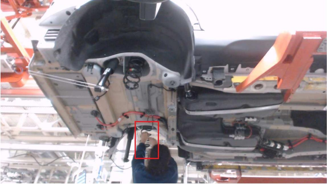
Figure 1.7: Occlusion of the spring during inspection of the underbody.
