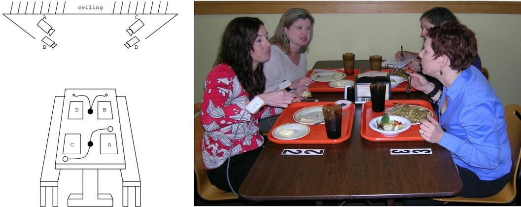
Figure 2.1: The table instrumented for data collection. Each participant wore a custom tethered device to track wrist motion.
