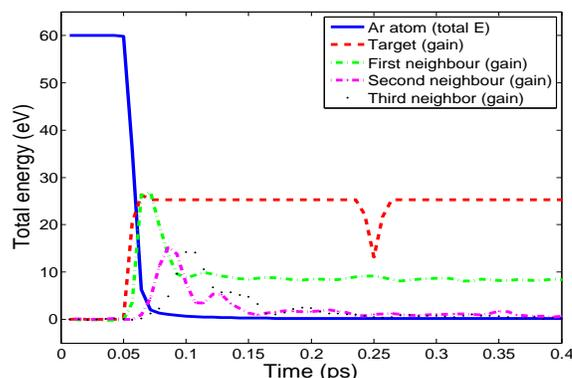
Figure 5: Energy exchange in Ar-SWCNT collision.
