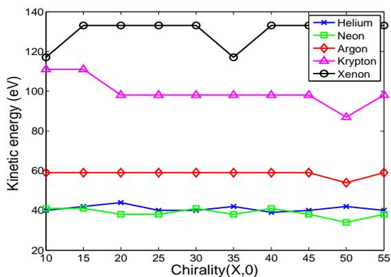
Figure 2: Minimum bond-breaking kinetic energy for SWCNTs with different chiralities .
