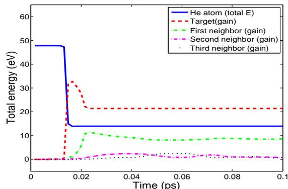
Figure 4: Energy exchange in He-SWCNT collision.
