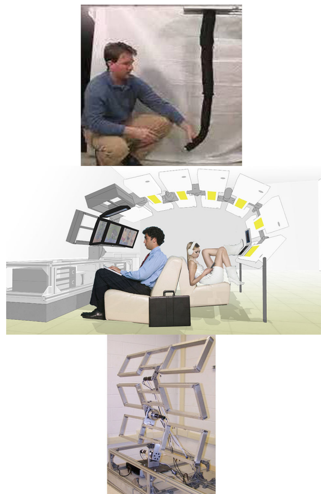
Fig. 2 An evolution of interactive robot technology in the AWE project from a linear form ( top ) previously developed and fielded by the authors, to a smooth surface ( center ) initially conceived for AWE, and to a hybrid of these two ( bottom ) in the final AWE implementation
