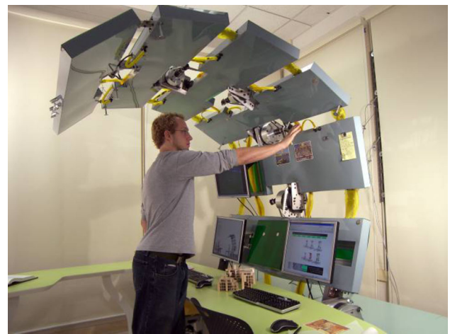
Fig. 10 Users fine-tuning AWE via IR sensors
