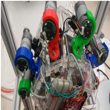
Fig. 3: Tendrill robot actuator package featuring nine DC motors all resting on load cells for tension sensing.
