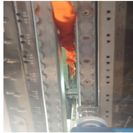
Fig. 14: Tendril robot penetrating gap between two racks.
