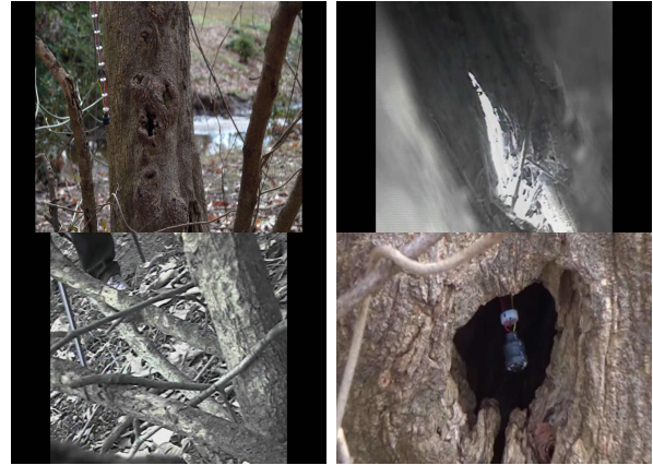
Fig. 10: Inspecting a dead tree through small knot hole. Top to bottom, left to right: increasing time.
