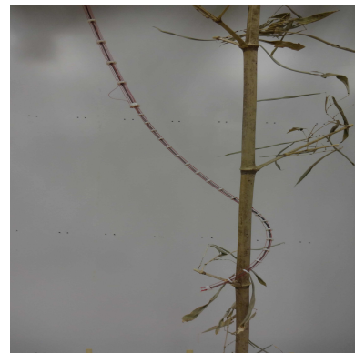
Fig. 1: Three section, spring-loaded concentric tube continuum robot with three tendons per section allowing local backbone extension and bending in all directions.
