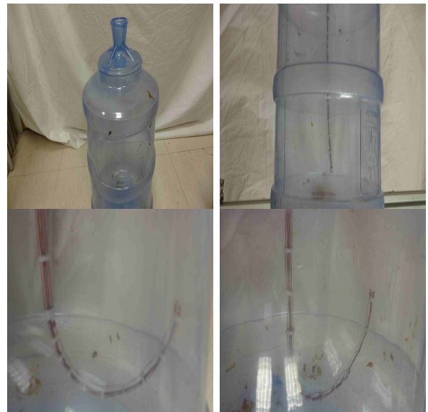
Fig. 8: Robot tendril backbone braced against environment. Top-left: Jug, Top-right: Tendril entering jug, Bottom-left: max unbraced bending, Bottom-right: Bending with bracing.
