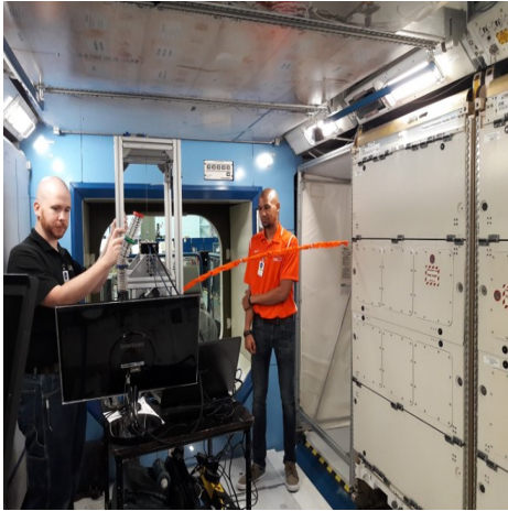
Fig. 12: Robot in Space Station mock-up environment. Tendril backbone has orange covering.
