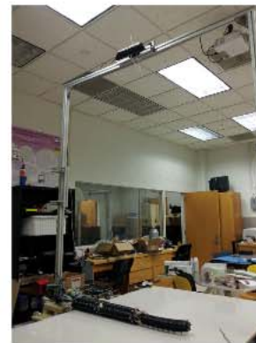
Fig. 1. Experimental set up with a table top OctArm, overseen by an overhead Microsoft Kinect
