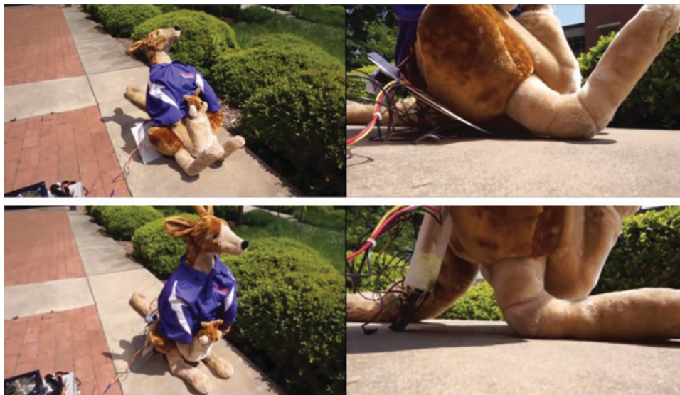
FIG. 13. Robot functioning as kangaroo tail. Top: Kangaroo unable to stand when tail loosened. Bottom: Kangaroo stands when tail stiffened. Color images available online at www.liebertpub.com/soro
