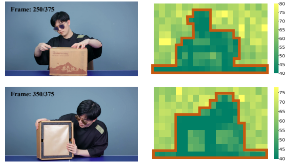
Figure 1. Patch PSNR heatmap of two frames in a 15s video when super-resolved by a general WDSR model. A clear boundary shows that PSNR is strongly related to video content.
