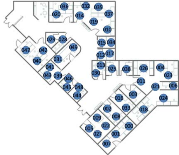
Fig. 8. Testbed consisting of 50 TelosB motes placed throughout 22 office and lab areas on the second floor of an office building. The device IDs range from 000 to 049.
