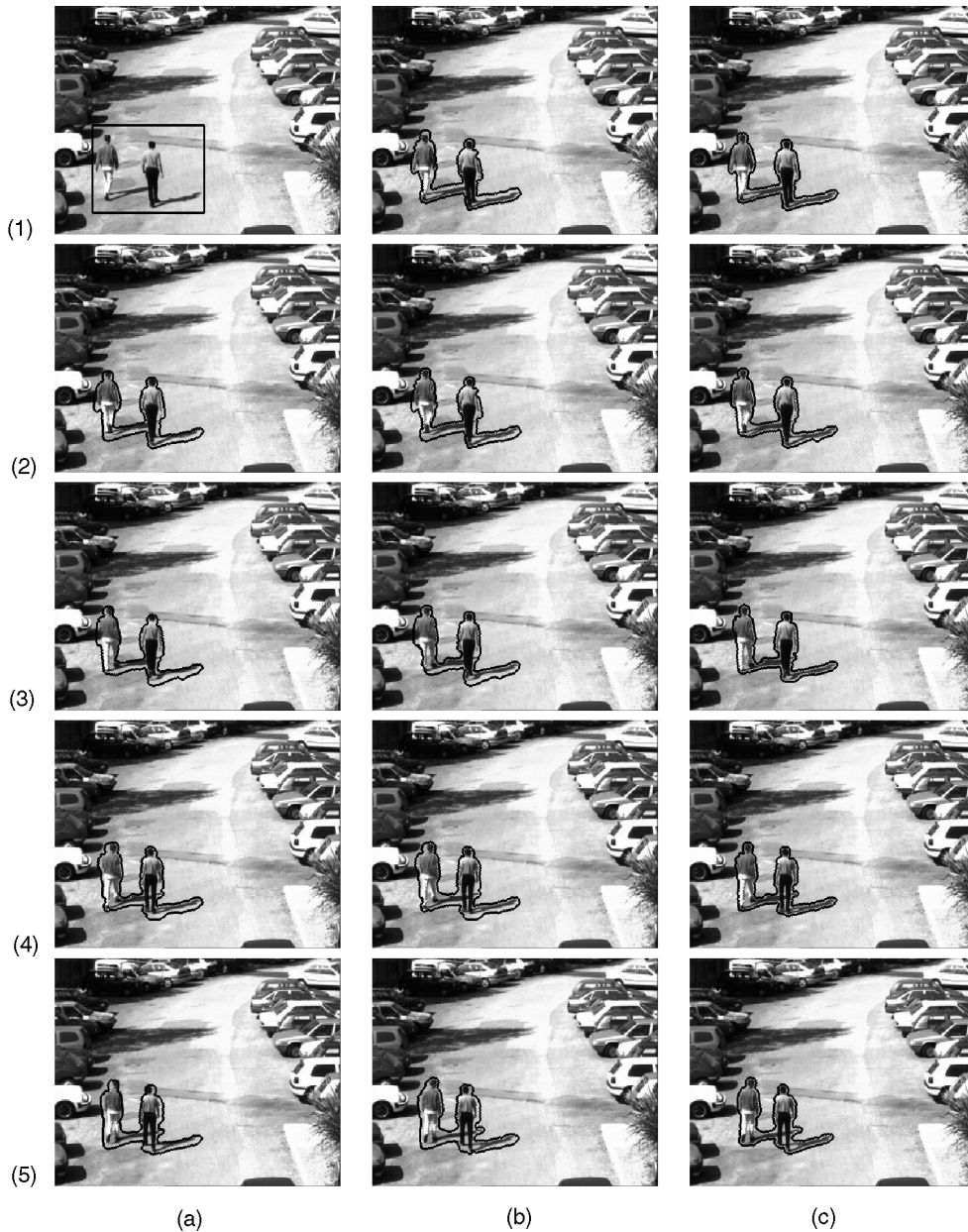
Fig. 13. Motion detection and tracking for Pierre and Imed sequence (1, 2, 3, 4, and 5). Front propagation algorithm: Hermes . (a) Initial curve, (b) motion detection result (between the current and the previous frame), and (c) tracking result. This sequence satisfies the constraints imposed by our approach. The background is smooth, while the consecutive object positions are overlapped. Besides, occlusions are not handled.
