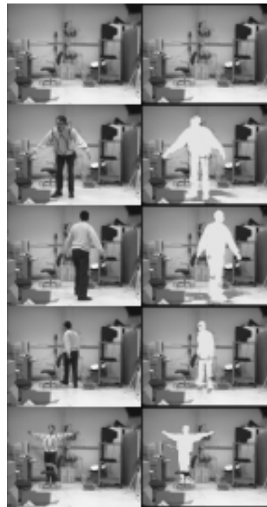
Figure 4. An example shows the result of our algorithm applying on a sequence of a person moving in an indoor scene. The scene, the left column is input sequence, and the middle column shows the output from our background subtraction (the foreground pixels are overlaid by light grey, the shadows are overlaid by dark grey, the highlights are overlaid by white, and the ordinary background pixels are kept as the original intensity.) The right column shows only foreground region after noise cleaning is performed.
