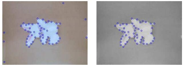
Fig. 4. LEFT: KLT features detected in the whole image. RIGHT: The subset of features that are located within the foreground region found by graph-based segmentation.
