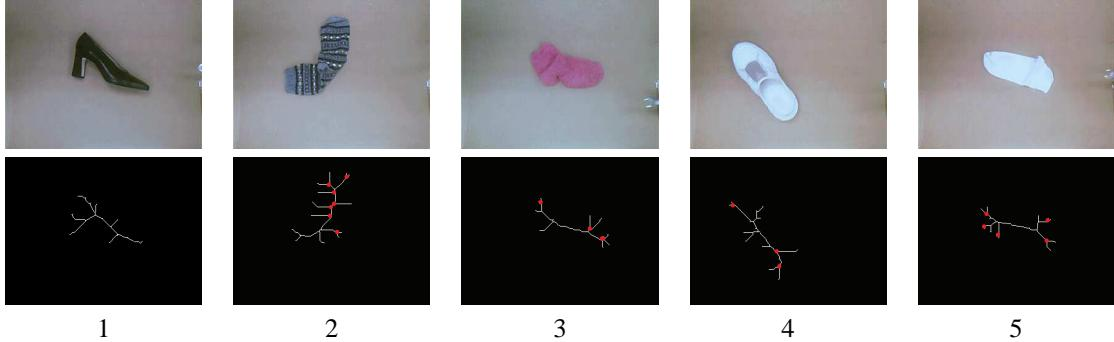
Fig. 12. TOP: Images of the individual objects gathered automatically by the system for the purpose of creating a database of objects previously encountered. BOTTOM: The final skeletons with revolute joints labeled.
