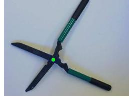
Fig. 9. Results of [3] on a pair of hedge clippers, with the green dot representing the revolute joint.
