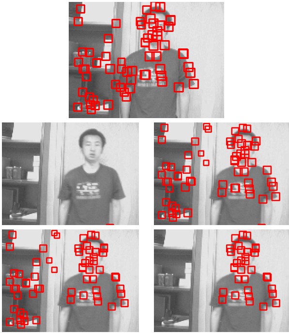
Fig. 4. Step-by-step results when the person and background have similar disparity. The images follow the same order as in Figure 3. The algorithm does not assume that the person is the closest object.
