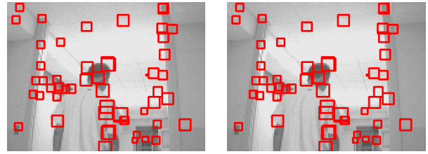
Fig. 2. Left and right images with features overlaid. The size of each square indicates the horizontal disparity of the feature. Since disparity is inversely proportional to depth, smaller squares are farther from the robot.
