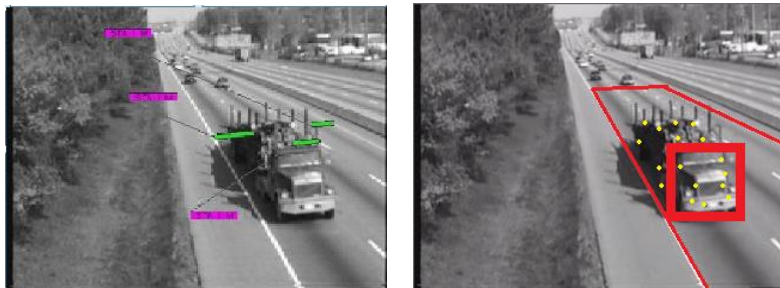
FIGURE 1: (a) A traditional video-based sensor relies on virtual detectors (green lines), thus resulting in over counting of trucks due to the triggering of multiple virtual detectors. (b) The Clemson video-based system correctly handles spillover, allowing the truck to be tracked as a single vehicle.
