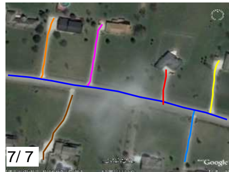
Figure 9.8: The results of urban road detection in sample satellite images. Centerlines of different roads are marked with different colors.
