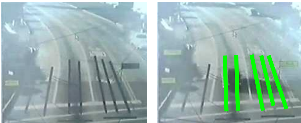
Figure 1.2: Shadow of a car incorrectly triggers a detection in neighboring lane.
