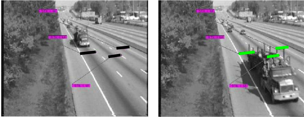
Figure 1.1: An example where large vehicles trigger multiple detection zones resulting in over counting. The output is from a popular commercial system (Autoscope). It should be noted that the commercial system is not designed to handle such a situation and it produces good results when the camera is placed high above the ground (40 feet or higher) with sufficient tilt angle.
