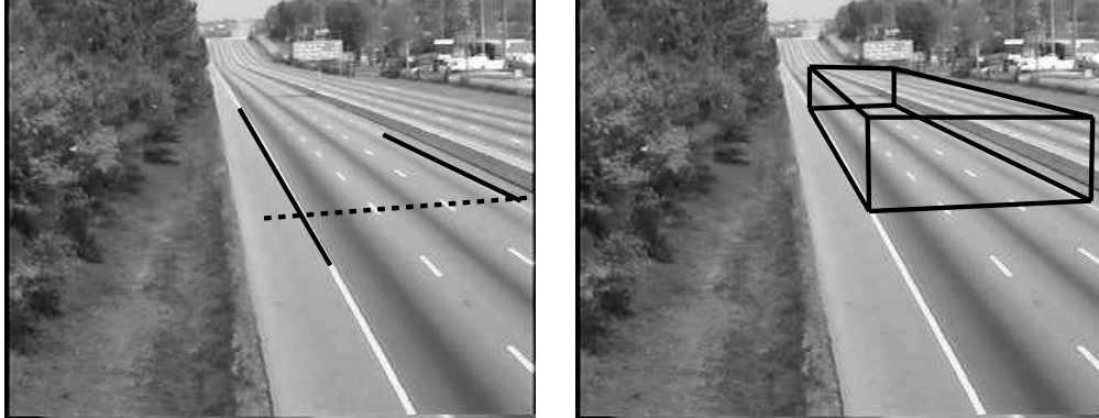
Figure 2.2: Manual camera calibration. LEFT: The user draws three lines, two along the edges of the road (solid) and one perpendicular to the direction of travel (dashed). The lines can be of arbitrary length. RIGHT: The 3D tracking zone is automatically computed.
