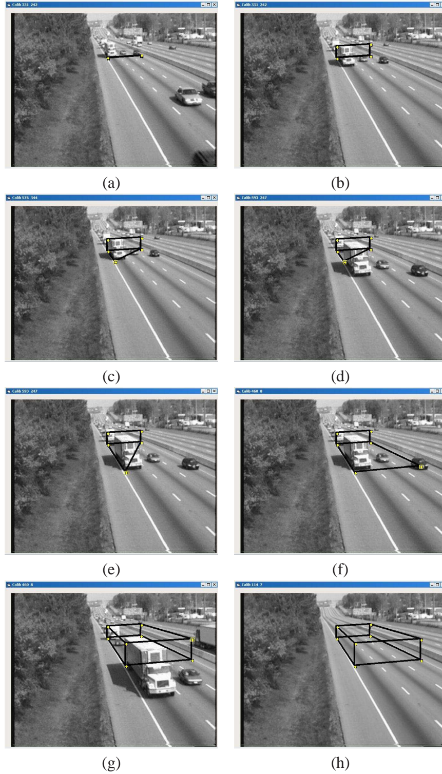
Figure 4.2: Camera calibration process for direct estimation of projective matrix.
