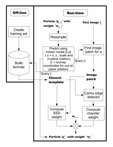
Figure 5.7: Block diagram of 'Isomap tracking with particle filter' algorithm for a single particle.
