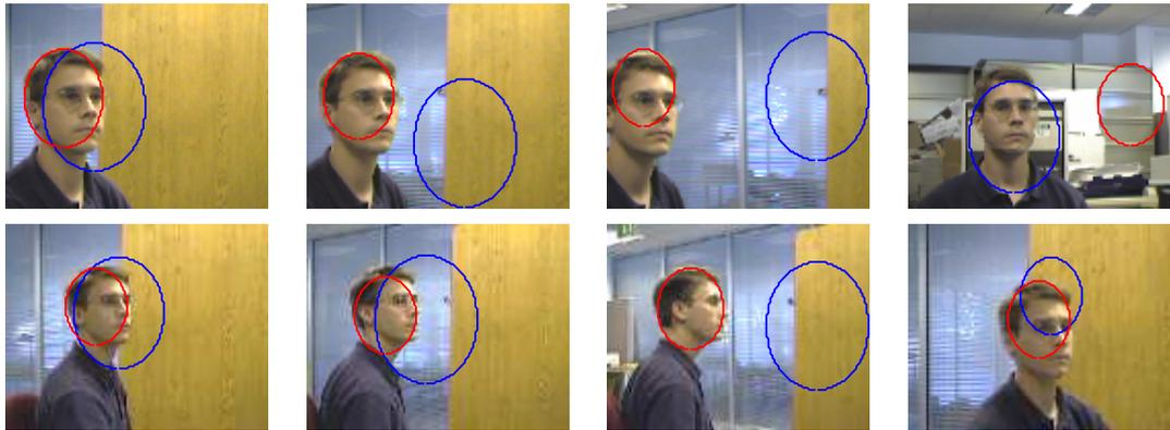
Figure 6.5: Tracking results for color histograms (blue) vs Haar histograms (red) for Sequence 1. Shown are frames 122, 125, 129, 146, 400, 407, 413, 465.
