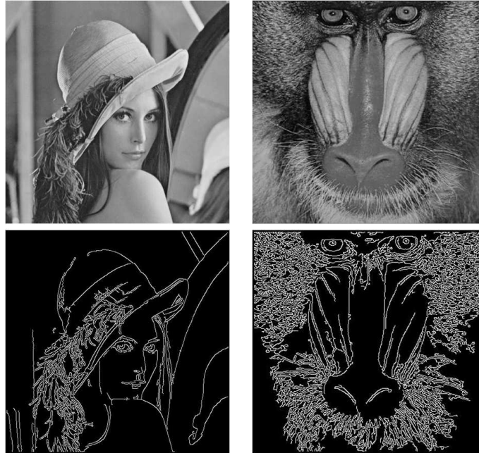
Figure 6.3: Typical inputs to and results of Canny edge detection. LEFT: Input “Lena” sized 1024 \times 1024 pixels. \sigma=1.0 , kernel size=5. RIGHT: Input “Mandrill” sized 1024 \times 992 pixels. \sigma=1.2 , kernel size=5.
