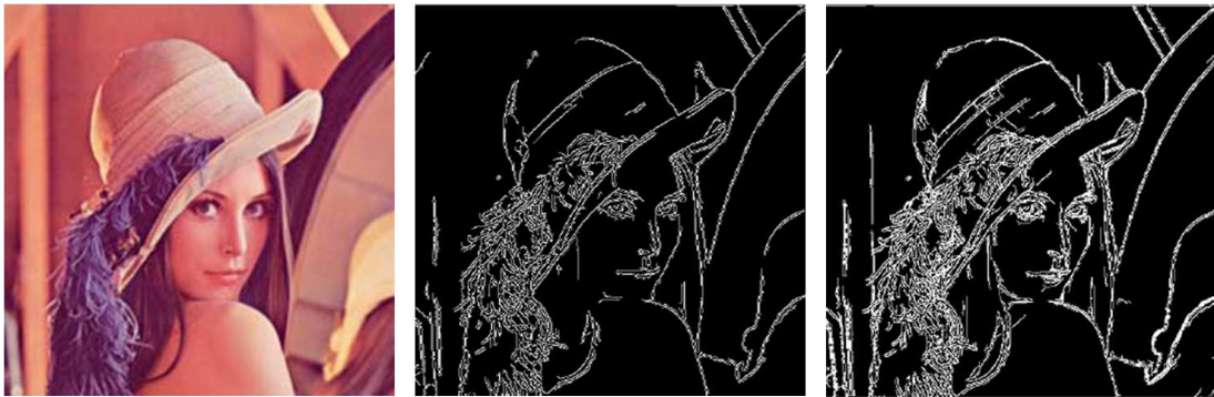
Figure 3.4: Comparing results of grayscale and color Canny edge detection. LEFT: Input image “Lena” of size 1024 \times 1024 pixels. CENTER: Output of Grayscale Canny edge detector with \sigma=0.8 , Gaussian kernel size = 5 \times 5 . RIGHT: Output of Color Canny edge detector with \sigma=0.8 , Gaussian kernel size = 5 \times 5 .
