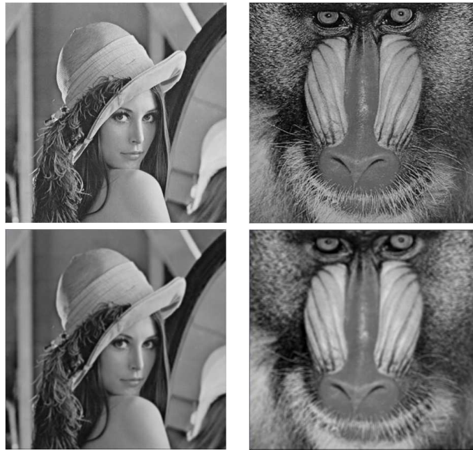
Figure 6.1: The results of 2-D Gaussian smoothing on standard input images. LEFT: Input “Lena” sized 1024 \times 1024 pixels. \sigma=1.0 , kernel size = 5. RIGHT: Input “Mandrill” sized 1024 \times 992 pixels. \sigma=2.4 , kernel size = 5
