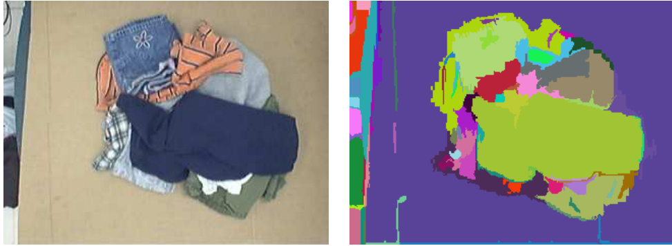
Figure 3.2: LEFT: An image taken by one of the overhead cameras in our setup. RIGHT: The results of applying the graph-based segmentation algorithm. Despite the over-segmentation, the results provide a sufficient representation for grasping an article of clothing.
