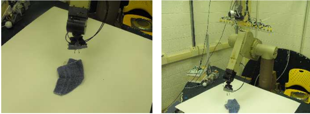
Figure 1.2: The robot system used for flattening a piece of clothing, in this case a washcloth: One PUMA manipulator and one Logitech Quickcam 4000.
