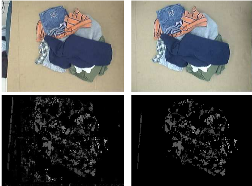
Figure 3.3: TOP: A stereo pair of images taken by the overhead cameras in our setup, showing the large amount of photometric inconsistency. BOTTOM: The disparity image obtained by SAD matching with the left-right disparity check (left), and the result after masking with the foreground and removing small regions (right).
