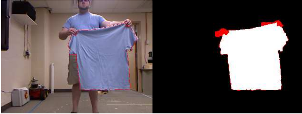
Figure 5.7: Left: Color image within a shirt sequence. Right: Segmentation of shirt from background while using the skin detector. White pixels represent foreground (shirt), black pixels represent background, and red pixels represent skin.
