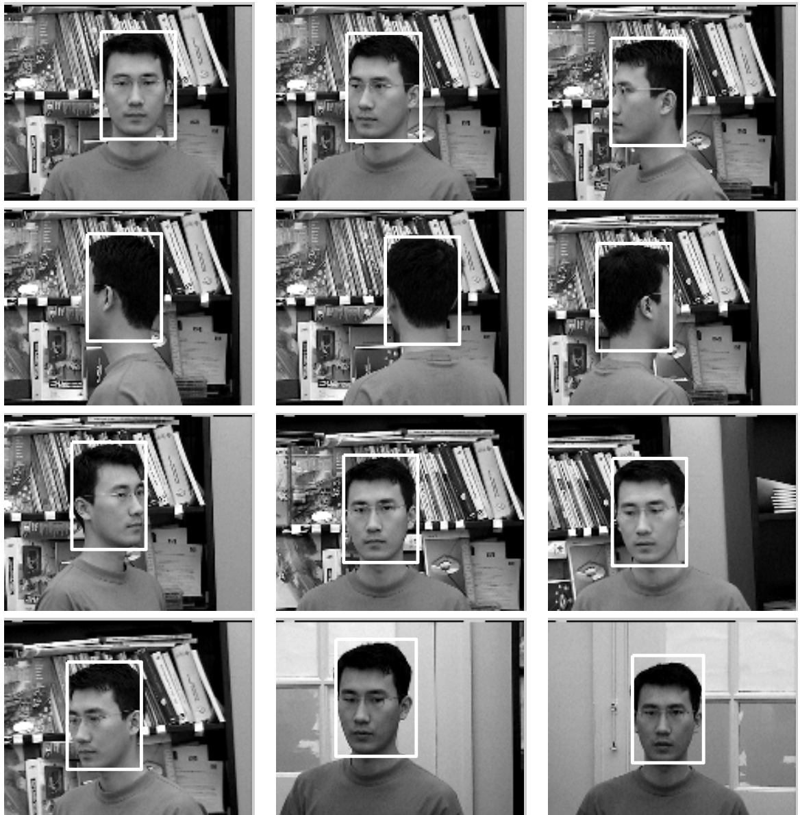
Figure 5.2: Tracking results of our algorithm on a sequence with cluttered background. Frame 10, 15, 20, 25, 30, 43, 51, 62, 164, 169, 197 and 239 are shown. The algorithm maintains a tight lock on the target in all the intermediate frames of the out-of-plane rotation.
