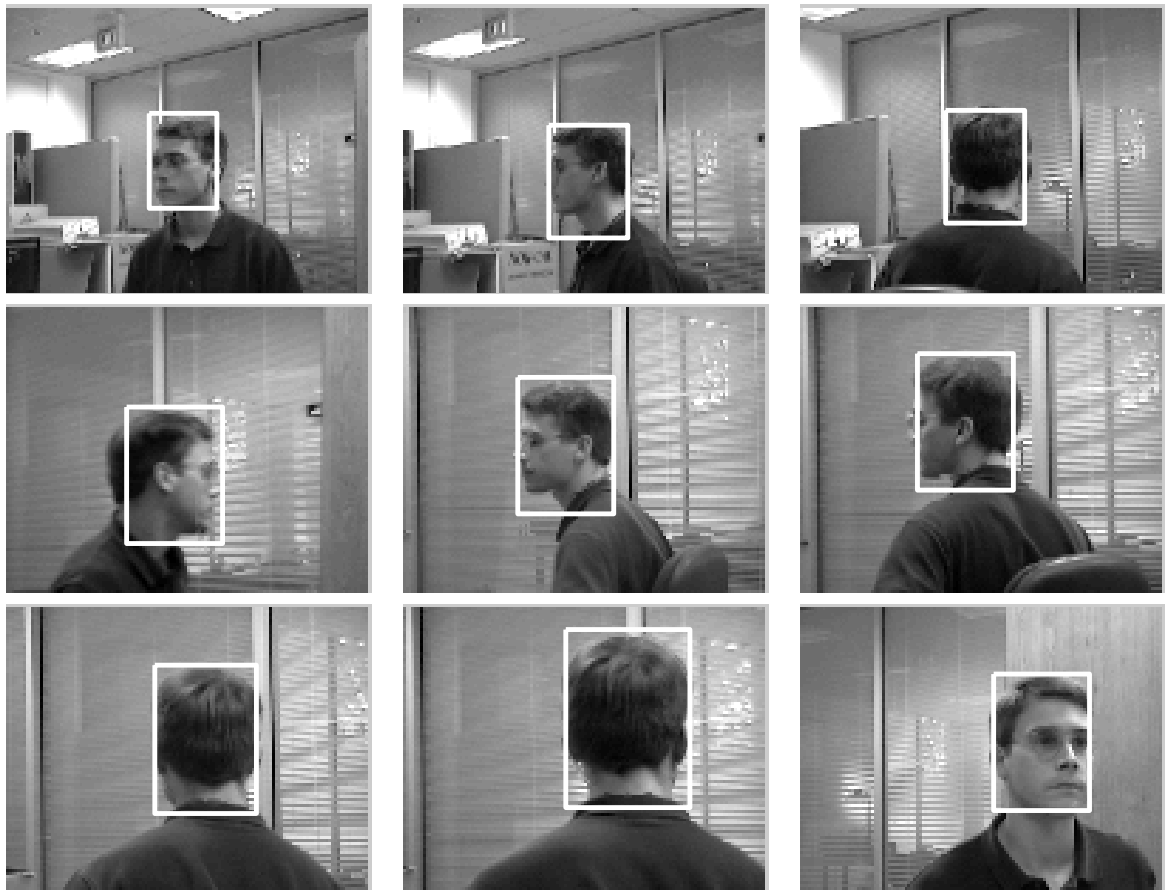
Figure 5.5: Tracking results of our algorithm on a sequence with untextured background. Frames 20, 25, 33, 44, 63, 67, 76, 81 and 102 are shown. The tracker is able to handle out-of-plane rotation, along with scale changes.
