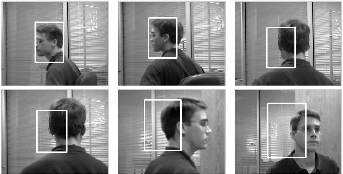
Figure 5.4: Tracking results of traditional template-based tracker on a sequence with untextured background. Frames 63, 67, 76, 81, 90 and 102 are shown. The tracker drifts away from the head due to out-of-plane rotation and loses the target completely after several frames.
