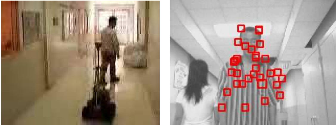
Figure 1.2: A typical example of person following. LEFT: A robot following a person. The person wears clothing with the same color as the environment. RIGHT: Feature detection and matching in order to extract the person.
