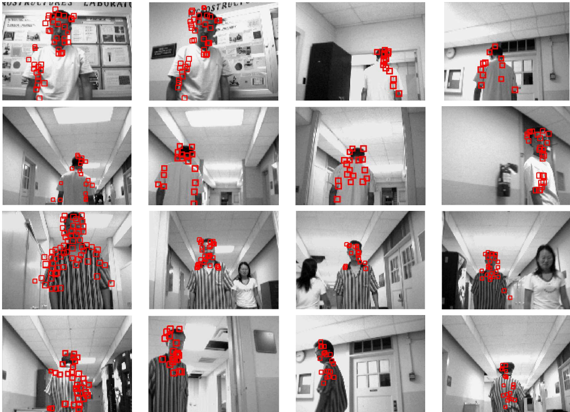
Figure 4.7: Sample images from a person following video. TOP TWO ROWS: Images taken by the left camera of the robot during an experiment in which the person wore a shirt with a similar color to the background. BOTTOM TWO ROWS: Images from an experiment in which another person walked by the camera.
