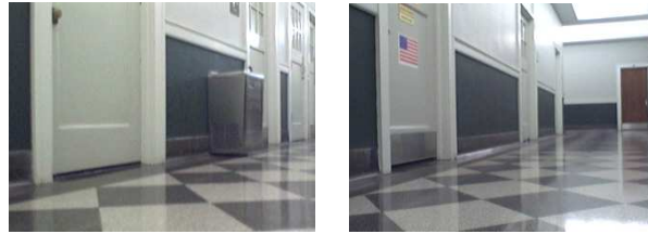
Figure 5.24: False negatives and positives. LEFT: One door is successfully detected, but another is missed due to lack of contrast along its bottom edge coupled with strong reflections on the floor; in addition a false positive occurs because of distracting horizontal edges. RIGHT: A dark door that is flush with the wall fails the concavity and bottom gap tests and hence is missed, while edges on the wall are erroneously detected.
