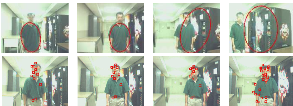
Figure 4.9: Sample images for comparison with color-histogram-based tracking. The results of the color-based algorithm (top) and our algorithm (bottom) in an environment with a textured background. The former loses the person, while the latter succeeds.
