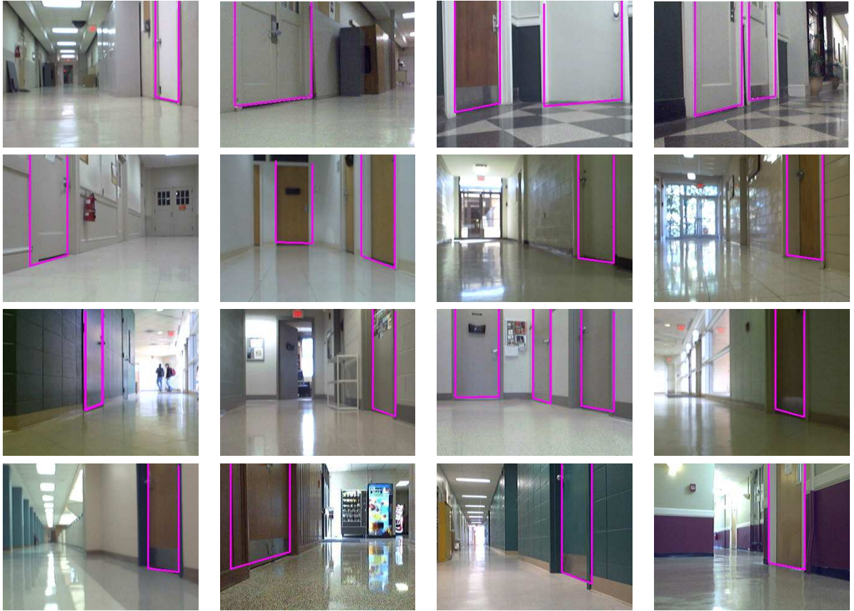
Figure 5.17: Examples of doors successfully detected by our algorithm. Note the variety of door widths, door and wall colors, relative pose of the door with respect to the robot, floor texture, and lighting conditions. Distant doors are not considered by the algorithm.
