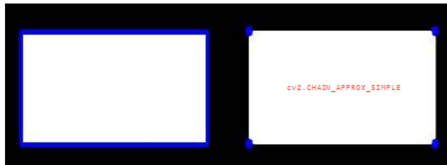
Figure 6. OpenCV Contour approximation method
