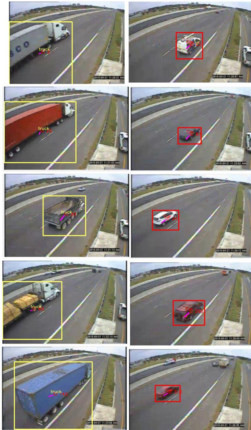
Figure 24. Demonstration of CNN classifier on SCDOT-recorded video
