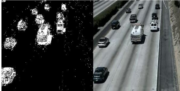
Figure 4. Background subtraction using Gaussian Mixture Model
