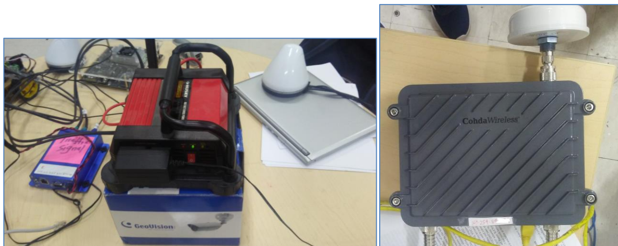
(i) Cohda MK5 On-board-unit (OBU) with power-supply (ii) Cohda MK5 Road-side-unit (RSU) Figure 7 OBU and RSU Used to Create a Connected Environment
