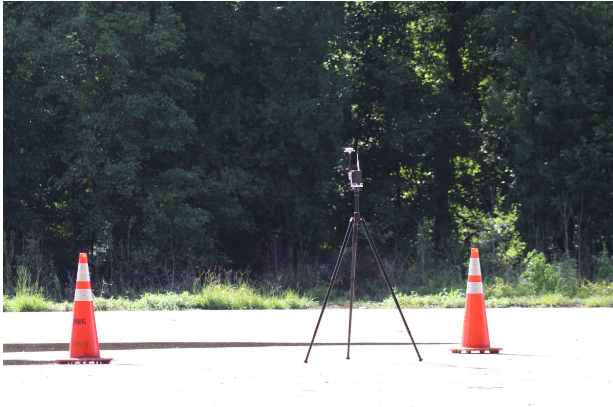
Figure 5.6: RTK ground station.
