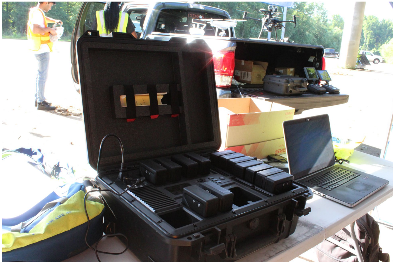
Figure 5.7: TB50 battery charging hub.
