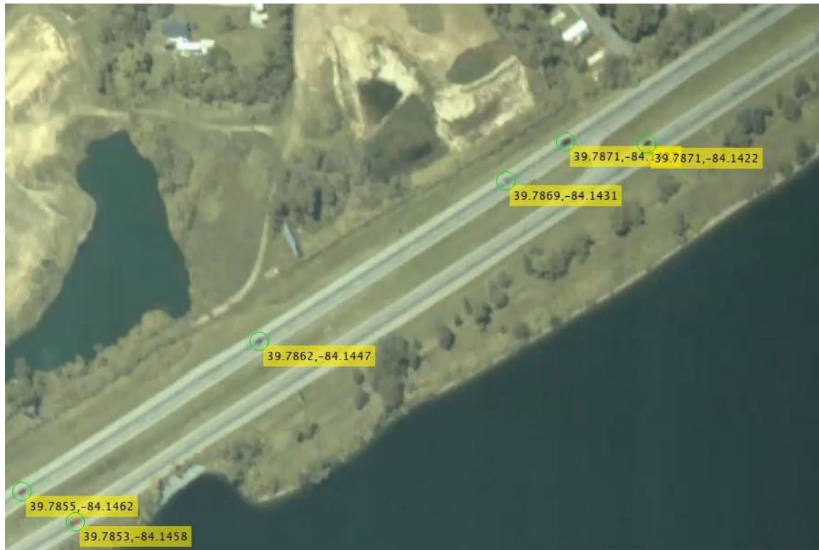
Fig. 8. Automatic identification of coordinates of detected vehicles
