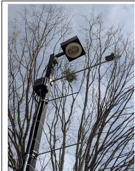
**Figure 1: Edge node mounted on a light pole.**
