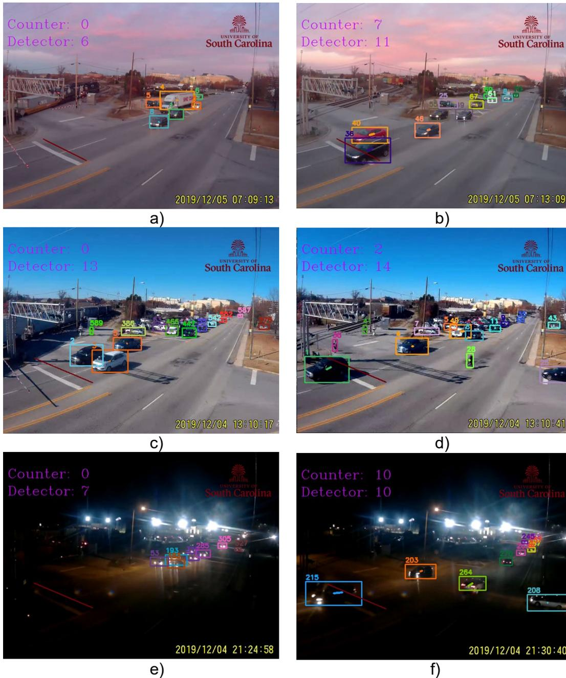
**Figure 4.2 Real-time vehicle detection and tracking system: (a)&(b) Morning condition during and after blockage; (c)&(d) Noon condition during and after blockage; (e)&(f) Night condition during and after a blockage**
