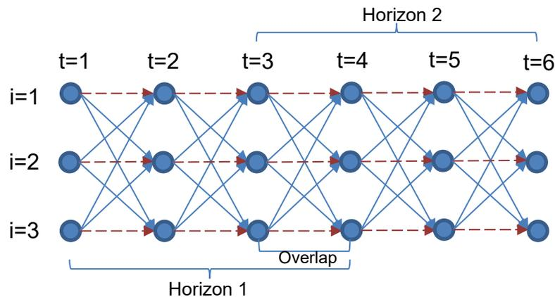
**Rolling horizon framework with  $i = 3$  and  $T = 6$ . Since the maximum single trip takes only one period, overlapping time is set to be 1**
