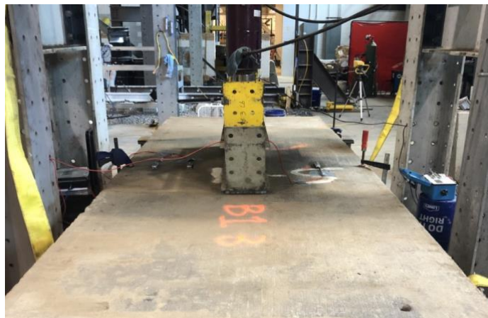
Figure 3.3 Laboratory testing of precast reinforced flat slab
