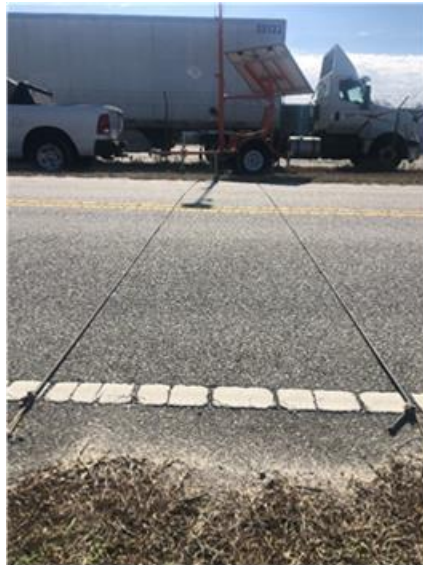
Figure 1: Pneumatic tubes deployed on Walter Price Road, Columbia, SC
