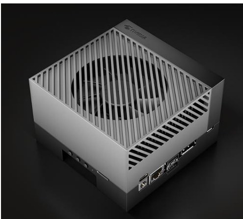
Figure 1.3 The edge device used in the work (Left: Nvidia Jetson AGX Orin; Right: Nvidia Jetson AGX Orin Core)
