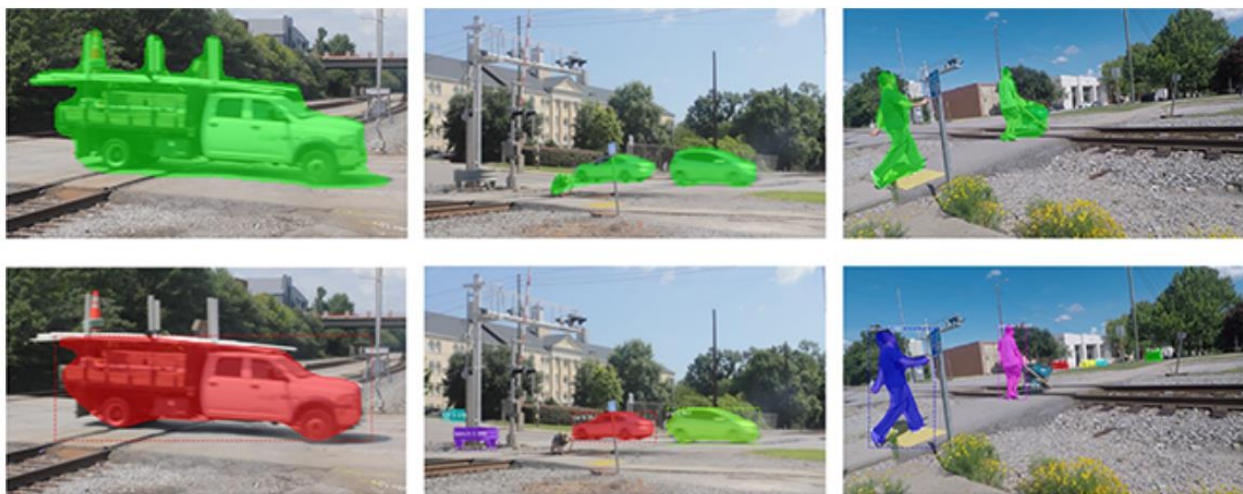
Figure 2.1 Differences between foreground segmentation and object detection (from top to bottom: foreground segmentation, object detection)
