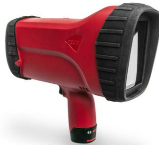
Figure 3 The handheld RetroSign GRX 554 retroreflectometer, used for measuring traffic sign retro-reflectivity during the study (TAPCO, 2024).
