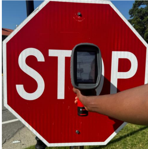
Figure 5 Shows measuring and recording the retroreflectivity coefficient of the Legend color of a stop sign in the study area
