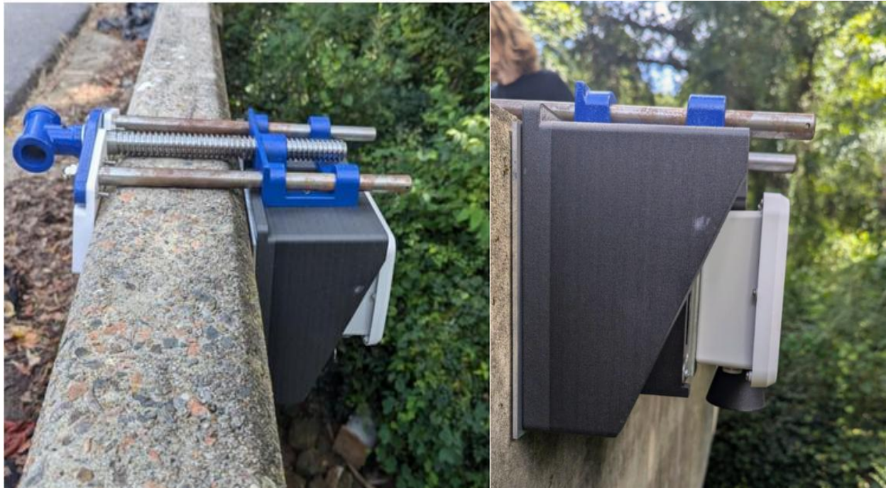
Figure 15: BridgeBox™ Custom Modified Vise
