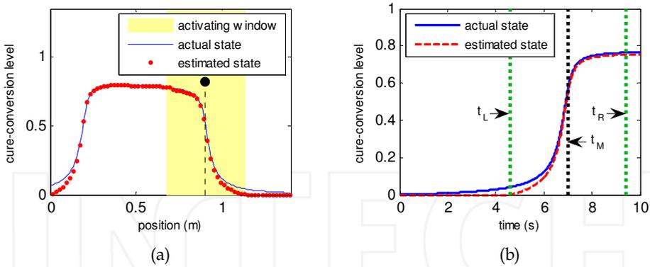
Fig. 9. (a) The distribution of the cure-conversion level along the target strip when the source is crossing the position ( $x=0.9m$ ) (b) The time history of the cure-conversion level for the position ( $x=0.9m$ )
