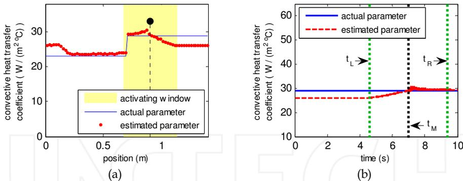
Fig. 11. (a) The distribution of the convective heat transfer coefficient along the target strip when the source is crossing the position ( $x=0.9\text{m}$ ) (b) The time history of the convective heat transfer coefficient for the position ( $x=0.9\text{m}$ )
