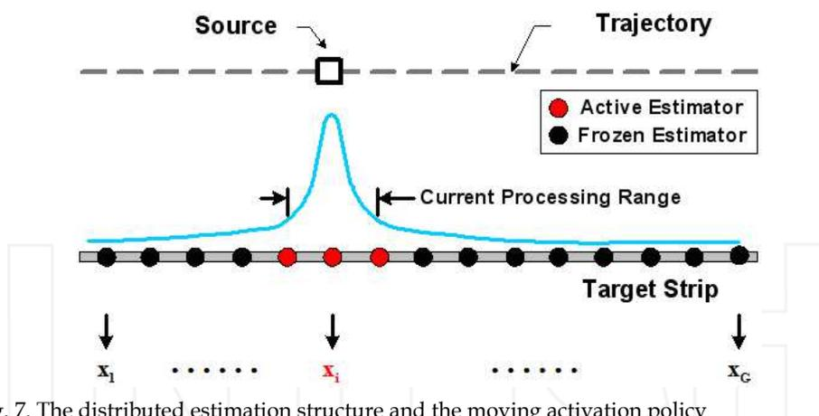
Fig. 7. The distributed estimation structure and the moving activation policy
