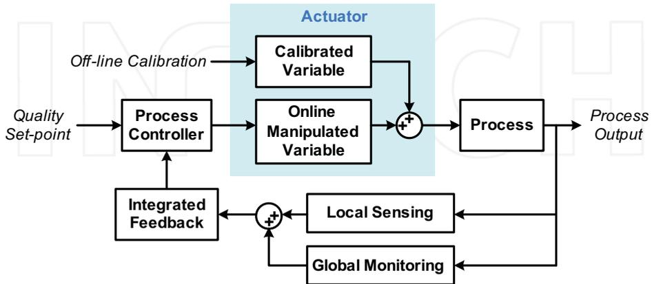
Fig. 4. The general output (temperature) feedback control structure
