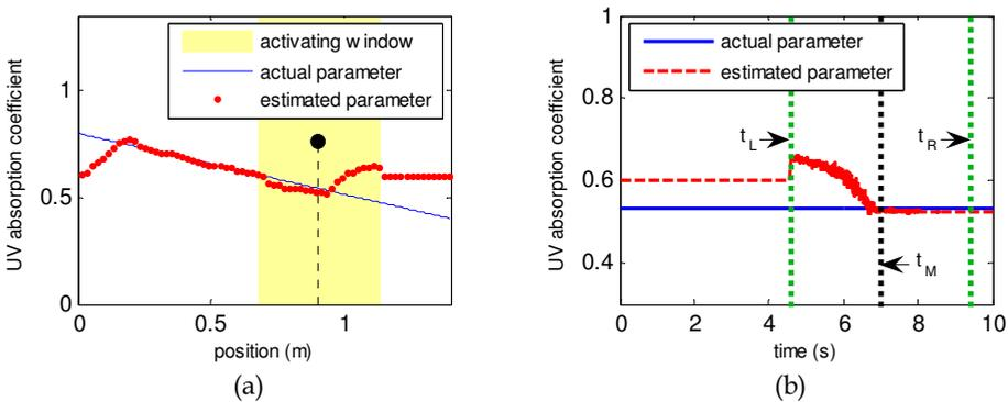
Fig. 10. (a) The distribution of the UV absorption coefficient along the target strip when the source is crossing the position ( $x=0.9m$ ) (b) The time history of the UV absorption coefficient for the position ( $x=0.9m$ )
