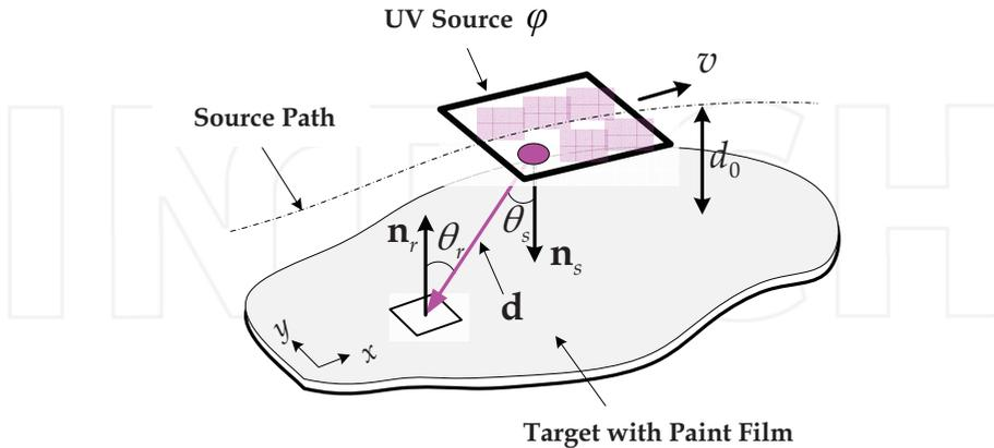
Fig. 2. The reduced schematic of a robotic UV curing process for a 2D target
