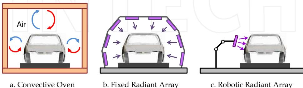
Fig. 1. Alternative automotive paint curing processes
