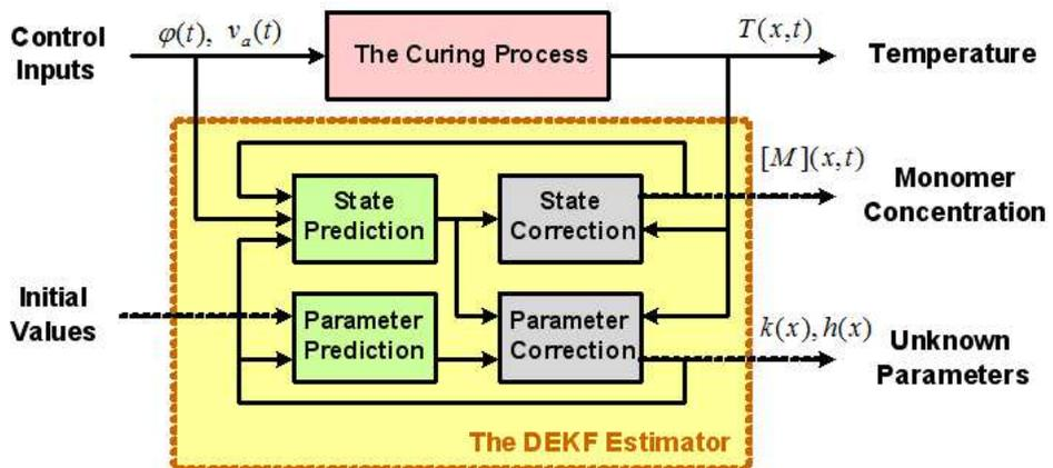
Fig. 6. The structure of the DEKF estimator
