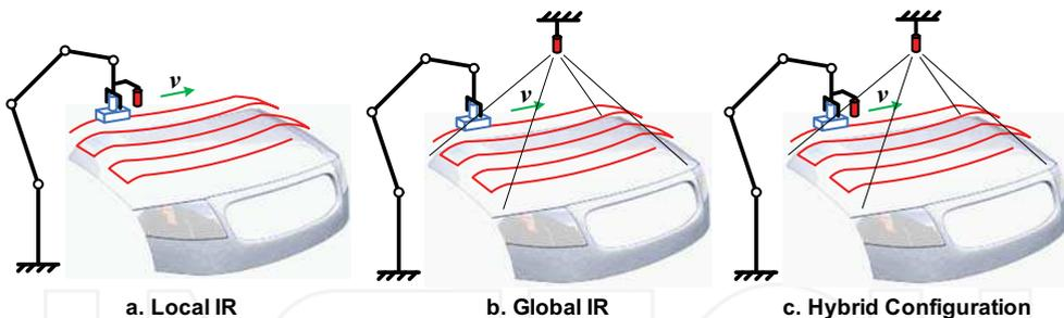
Fig. 3. Alternative temperature measurement configurations through IR cameras
