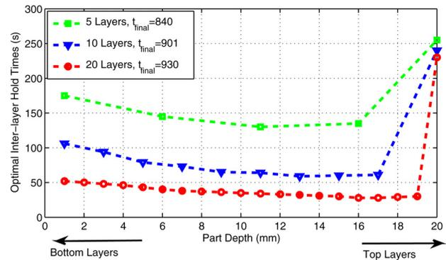
**Fig. 7 Optimal interlayer hold times for three cases**
