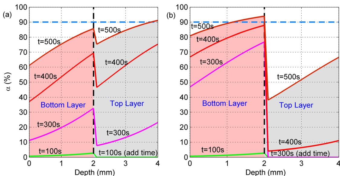
**Fig. 4 In process cure level distribution for a two-layer part with (a) early layer addition (at  $t = 100$  s) and (b) late layer addition (at  $t = 300$  s)**
