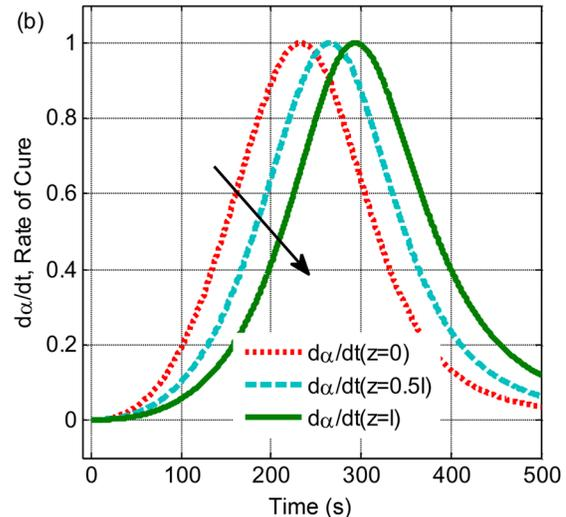
Fig. 2 (a) Propagation of the normalized rate of cure and the cure level at the bottom of the layer ( $z = l$ ); (b) Propagation of the normalized rate of cure in a layer at three different locations. (The normalization is with respect to the maximum value.)
