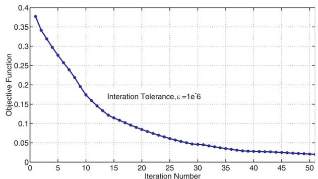
Fig. 11 Convergence of computational algorithm: Optimal cost for ten layers
