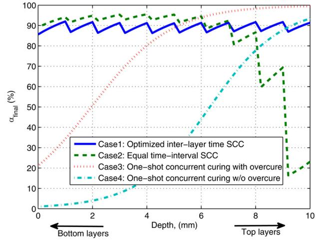
**Fig. 6 Achieved final cure level profile with SCC and one-shot curing**
