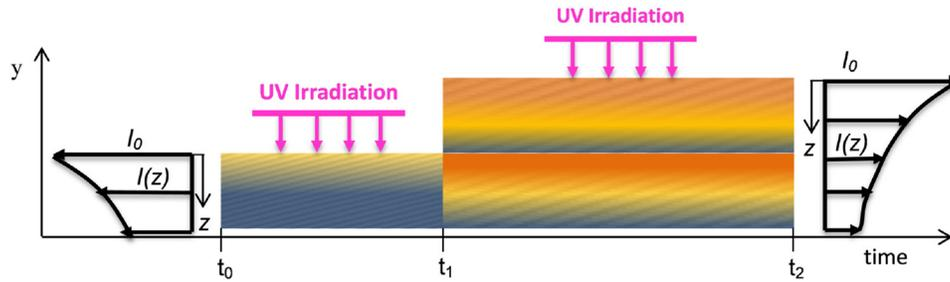
**Fig. 3 UV attenuation in a layer-by-layer process (y-axis is used to indicate the direction of part thickness increment as layers add on whereas z-axis indicates the direction of UV attenuation)**
