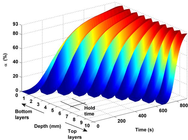
Fig. 8 Cure level profile with optimized SCC
