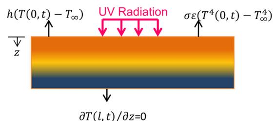
Fig. 1 Schematic of a UV curing process
