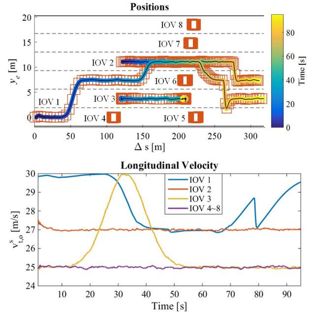
Fig. 8. States of the IOVs in a highway scenario. Top: relative positions, Bottom longitudinal velocities.
