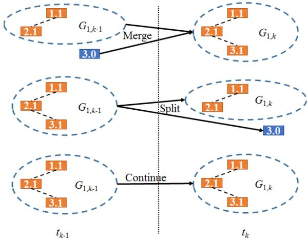
Fig. 2. Illustration of object vehicle group behaviors (number before dot is vehicle index, number after dot is group index, 0 means no group).
