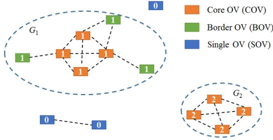
Fig. 4. Illustration of the DBSCAN grouping results ( $\mu = 4$ ). The edge means there is density-connection between the IOVs. Only the group index of each IOV is shown here. 0 means the IOV is SOV with no group index.
