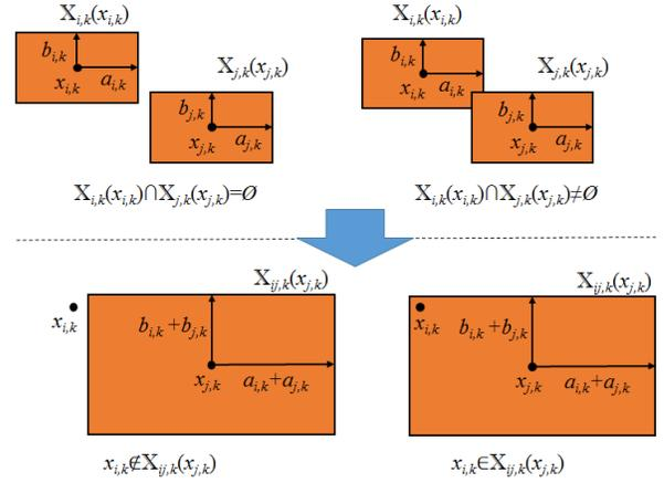
Fig. 3. Example of the collision condition for two IOVs with rectangular shape description in 2D ( $a$  is half length and  $b$  is half width).
