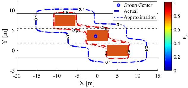
Fig. 5. Illustration of the OVG distribution contour in a 2D position space. The position states of the three IOVs are assumed to be Gaussian distributed.  $a = 0.1$  and  $a = 0.9$ . contours shown. Solid probability contours are calculated by (29) while the dash contours come from (30).
