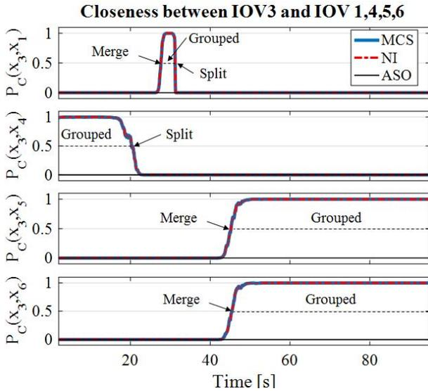
Fig. 10. Closeness between IOV 3 and some of the other IOVs under the Monte Carlo Simulation(MSC) method with 100000 samples, numerical integration (NI) method, and the approximation method for small-sized object (ASO).
