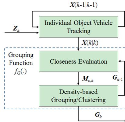
Fig. 1. Object vehicle grouping framework.
