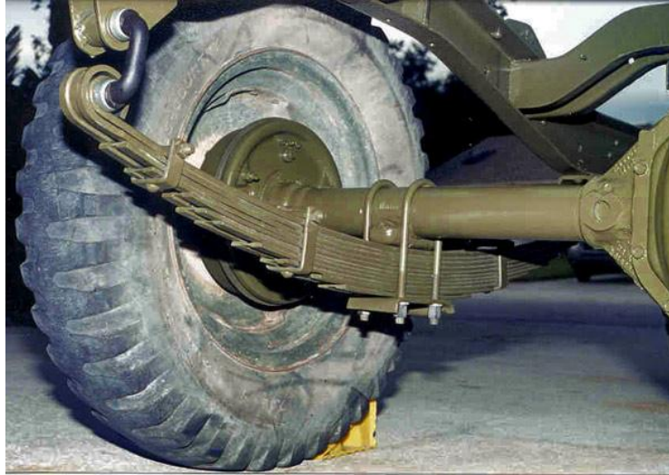
Figure 6 Longitudinal leaf spring used in Jeep (8)
